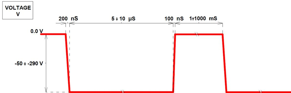
Fig 2. Typical Voltage Curve of the pulses that will be used in upcoming experiments. Next step will be pulse duration reduction down to 2  $\mu$ s, while increasing the peak voltage (up to -700 V).
